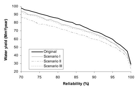
Figure 3. Yield – reliability curves for the original situation and for the three reference scenarios. The curves refer to the summation of the yield in the 15 largest reservoirs of the Salgado basin.
