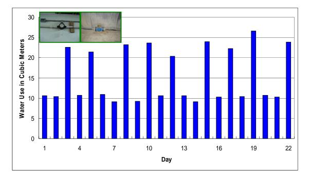
Figure 8 Typical Daily Water Use and Installed Flowmeters at Participating Layers Farm
