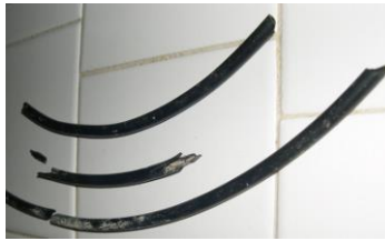
Figure 4: Portion of capillary tubes coming from the same initial piece with localized anti-oxidant fault
