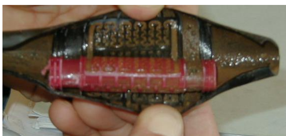
Figure 8 : Particles deposit in a GR dripper
