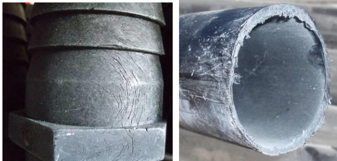
Figure 6: moulding homogeneity default on a fitting and heterogeneous wall thickness of a PE pipe (90mm)
