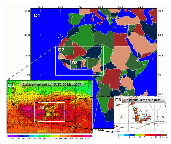
**Figure 2**. WRF forecast domains for the operational modeling system, with example forecast products on the two inner grids. The grid increments on D1, D2, and D3 are 40.5, 13.5 and 4.5 km, respectively. The forecasts are 48 h in duration on D1 and D2, and 36 h on D3.
