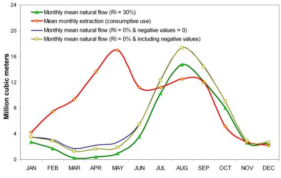
Figure 3. Natural flow and monthly mean consumptive use from 1982 to 2002.
