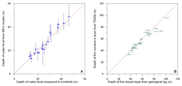
Fig. 2: Comparison of the geometry of aquifer obtained by geophysical and by invasive methods. A. Water level. B. Bottom of aquifer.
