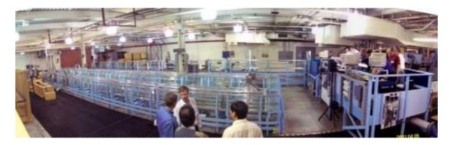
Figure 6. Model canal in Reclamation's Hydraulics Laboratory
