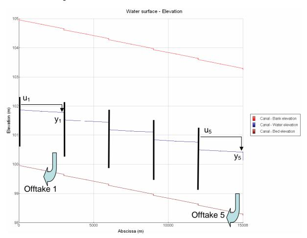
Figure 1. Schematic longitudinal view of the canal test
