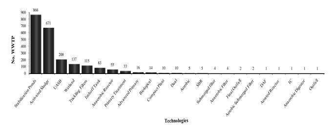
Figure 1 Technologies used in wastewater treatment in LAC
