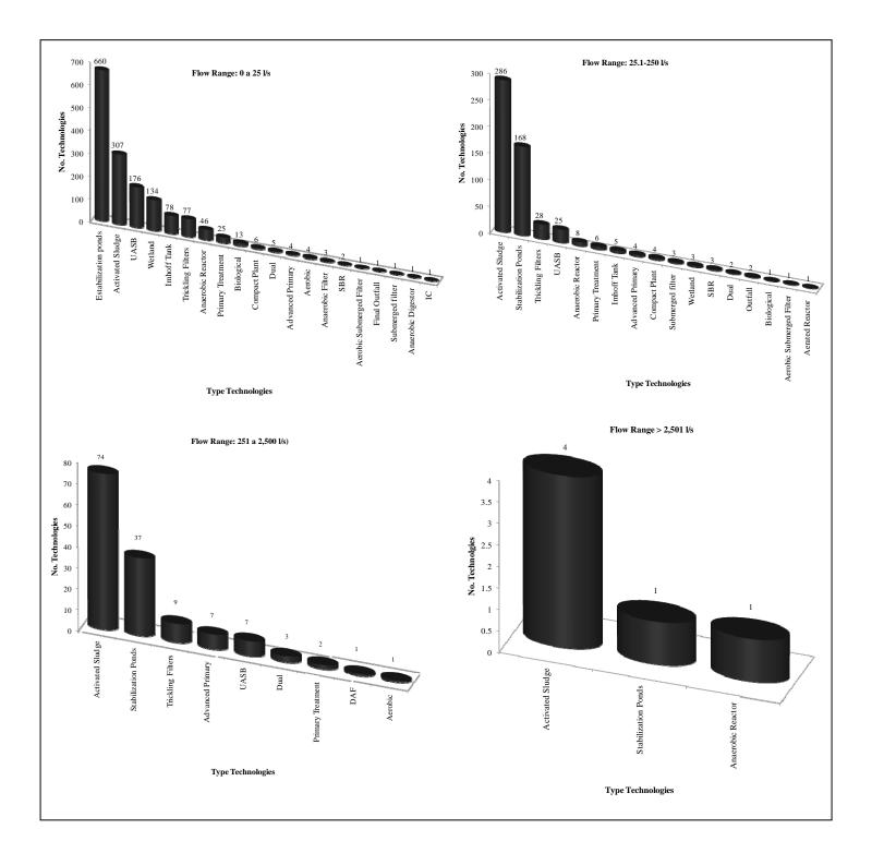
Figure 2 Distribution of the technologies used in flow rate interval in LAC
