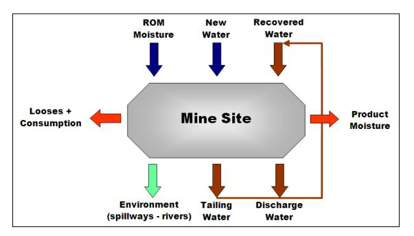
Figure 5: Simplified schematic mine site water balance (Rocci, 2009).
