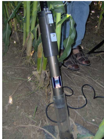
Fig. 4 – Tube for insertion of the transparent tube and endoscope BTC Minirhizotron Camera Systems, Évora University
