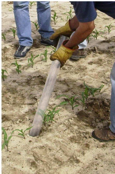
Fig. 4 – Tube for insertion of the transparent tube and endoscope BTC Minirhizotron Camera Systems, Évora University
