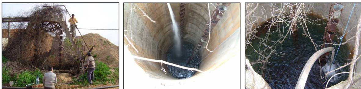
Figure 11 – Injection test developed in the “nora”: water levels at the beginning and at the end of the test
