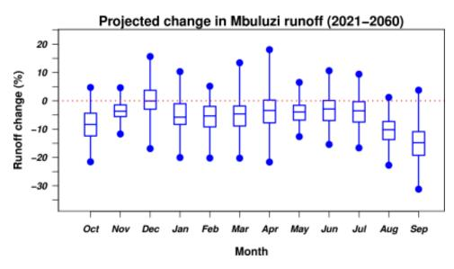
Figure 10: Projected runoff change in the Mbuluzi catchment. The box plots show the 95% confidence interval extending from the circles, which show the 2.5% and 97.5% quantiles.
