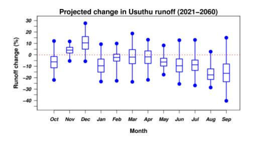
Figure 6: Projected runoff change in the Usuthu catchment. The box plots show the 95% confidence interval extending from the circles, which show the 2.5% and 97.5% quantiles.
