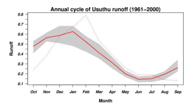
Figure 5. Observed and simulated streamflow in the Usuthu Catchment during verification
