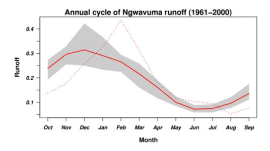
Figure 4. Observed and simulated streamflow in the Ngwavuma Catchment during verification
