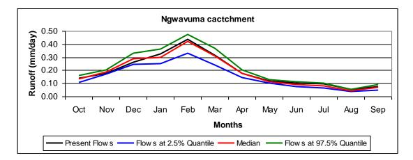
Figure 13: A comparison between present and future flows at the 2.5%, median, and the 97.5% quantiles runoff change in the Ngwavuma catchment
