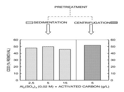
**Figure 2.** Influence of the application of Coagulation + CAP in COD removal of supernatant of Sedimentation and coagulation. Experimental conditions:  $pH_o=7$ , 0;  $COD_o=6$ , 9 g/L.
