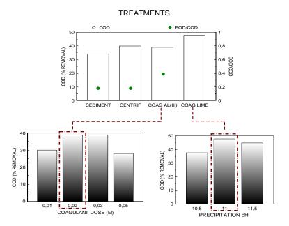
**Figure 1.** Influence of the pre-treatments in COD removal. Experimental conditions:  $pH_0=8$ , 3; COD<sub>0</sub> =10, 4 g/L.
