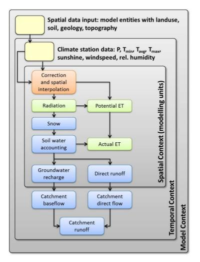
Figure 4: shows a diagram of the model structure
