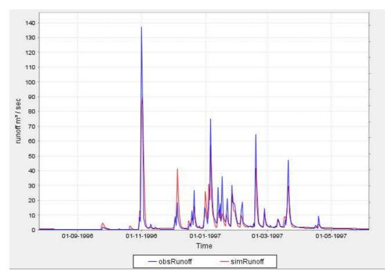
Figure 6: Observed and simulated runoff for the 1997 hydrological year.
