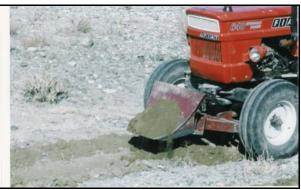
Fig 6: Ditcher, specialized instrument for ditch making Figure 6: Figure 5: Pit Maker for making pits in ditches
