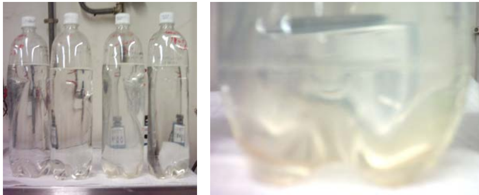
Figure 6 SORAS test and a detail of the arsenic residue after sun exposure period
