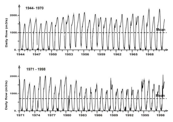
Fig. 3: Recorded natural flow of river Niger at Niamey for periods 1994-69 and 1971-98 (processed from raw data obtained from NBA)
