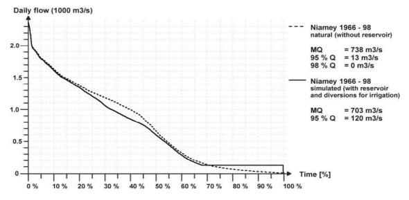
**Fig. 7:** Duration curves of daily flow of River Niger at Niamey (natural and simulated for a required minimum target flow of 120 m<sup>3</sup>/s)
