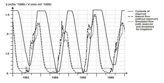
**Fig. 6:** Excerpt of simulation: contents of reservoir and corresponding flow of river Niger at Niamey for a required minimum target flow at Niamey of 120 m<sup>3</sup>/s
