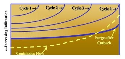
Fig. 5: Surge irrigation: Water percolation in surge and continuous flow
