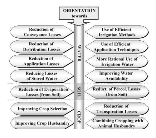
Fig. 2: Water conservation methods used in agriculture, directed either towards loss reduction or increase in efficiency of water use
