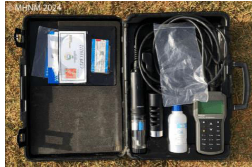
Hanna multiparameter used for in situ measurements
