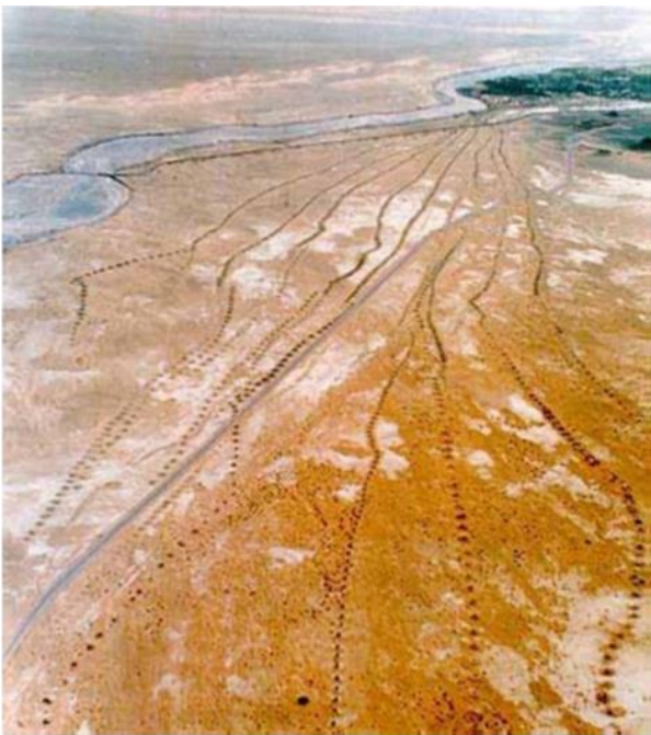
Photo of the khattara system in the Tafilalet Valley (www. Water history. org)
