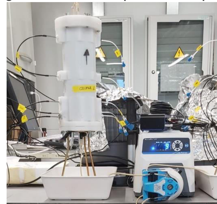
Figure 2. Soil-column experiment set-up.
