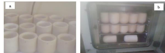
Filters drying at room temperature after pressing (a) and in the oven at 105 \pm 5 °C (b)
