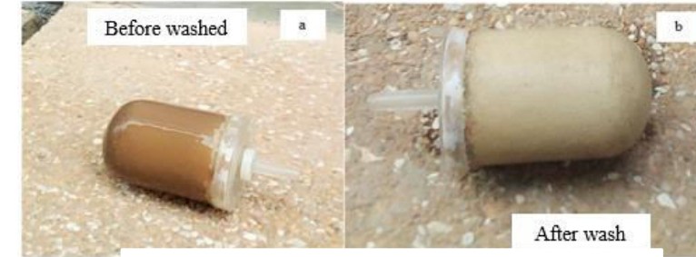
Filters after 8 weeks continuous operation
