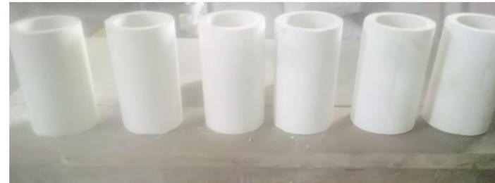
Plaster of Paris (POP) mould used in forming the filters
