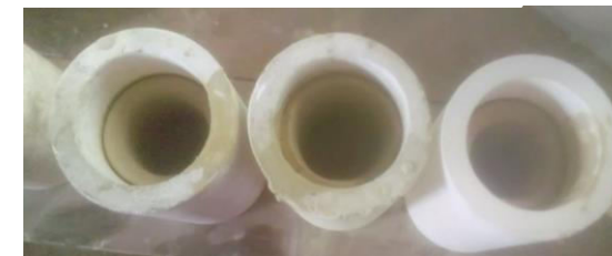
Formed filters ready for pressing
