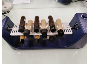
Batch experiments (20 mL) CECs concentration: 10 µg/L
