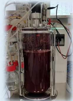
Cultivation – Stirred tank bioreactor 4 L* 30°C/100 rpm/7-days
