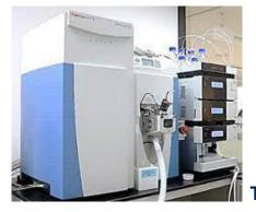
Liquid chromatographyhigh resolution mass spectrometry (LC-HRMS (Orbitrap-MS)
