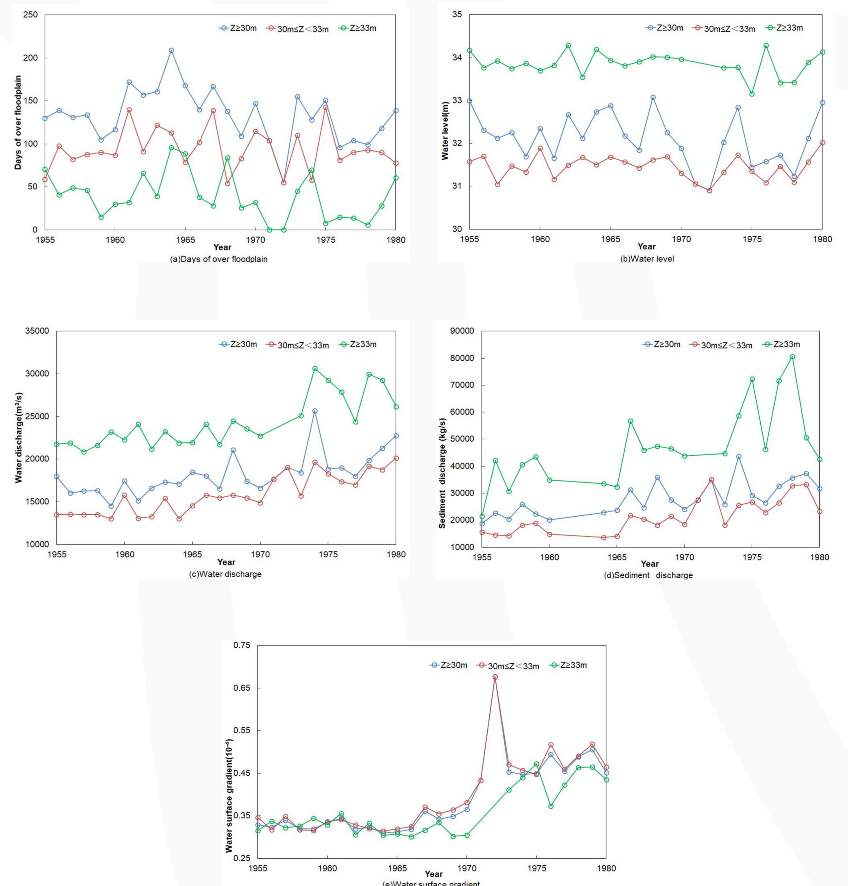
Figure 1 Hydrological Parameters of Shatanzi Cutoff River Section under Different Water Levels over Years
