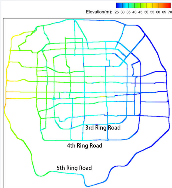
(a) Measured elevation of major roads
