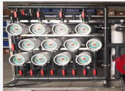
Brackish water membrane separation treatment equipment
