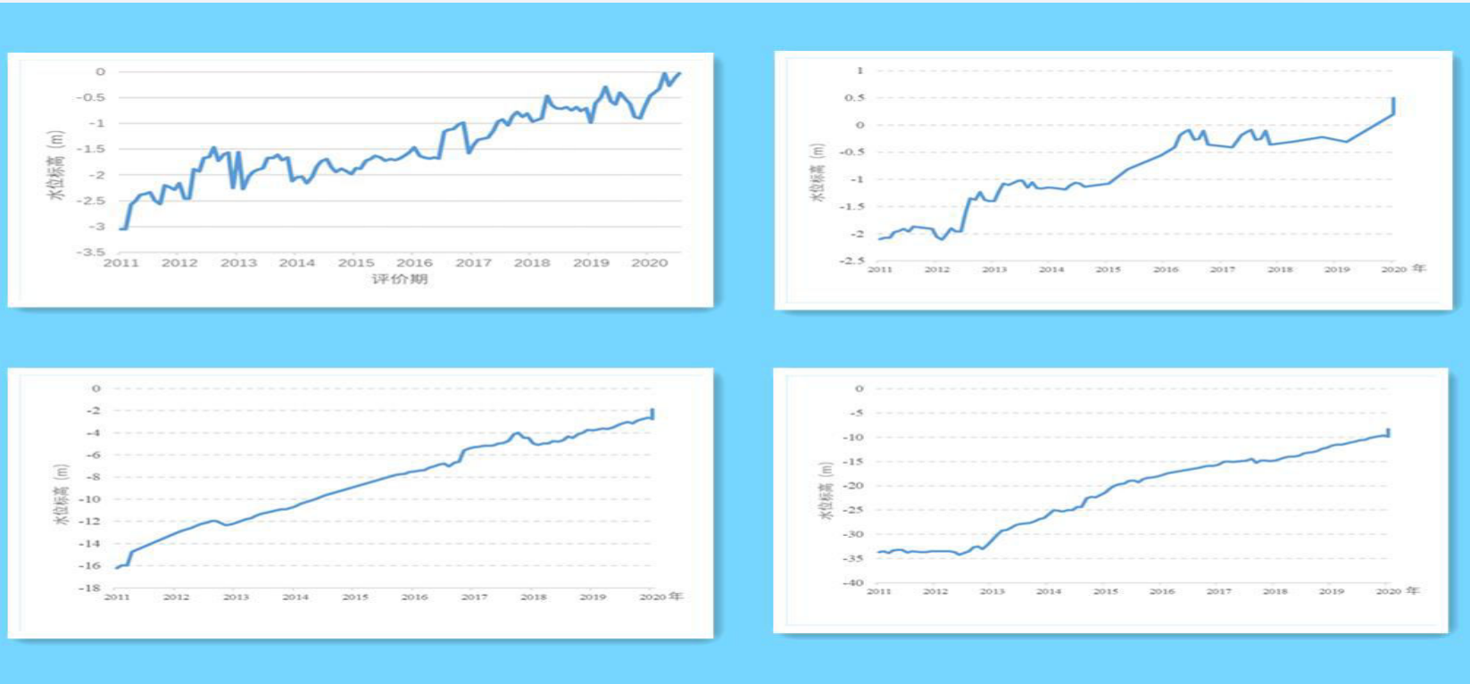
Longitudinal Change Curve of Groundwater Level in Typical Monitoring Wells of the Second to Fifth Deep Confined Aquifers
