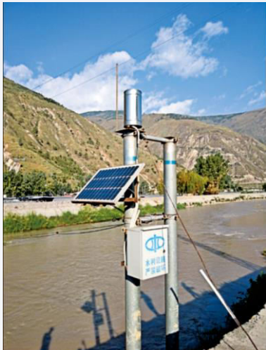
Automatic rain-gauge station
