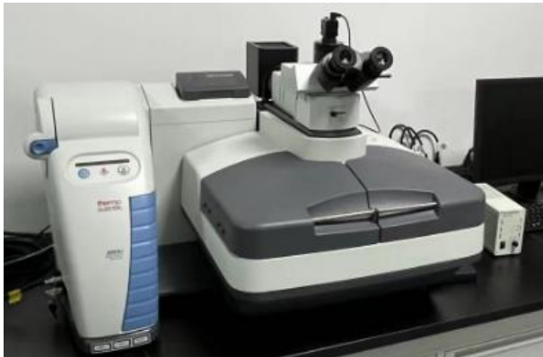
Microplastics testing equipment Microscopic Raman Spectrometer
