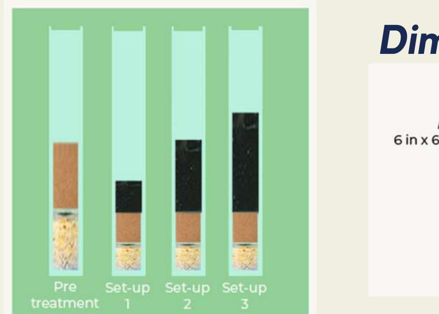
The collected water sample passed the sand and gravel filtration and the effluent were collected and tested and then the water sample passed through the three set ups which were consists of the different height of the activated carbon and also have the sand and gravel on it.
