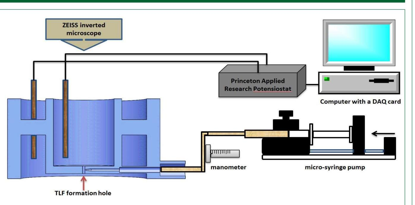
The MSC is filled with the surfactant solution and using the syringe pump and Hamilton micro-syringe, the oil phase is injected into the system. The
