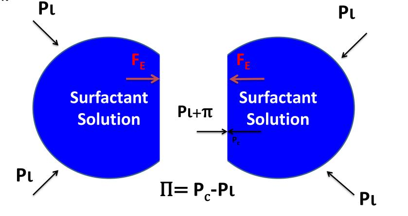
□ The concept of Force Balance and disjoining pressure in TLFs
