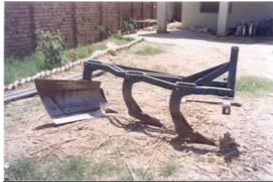
Fig 5: Ditcher, specialized instrument for ditch making
