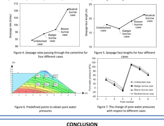
The change in seepage rate at centerline and the seepage face length are presented in Figures 4 and 5. The predefined points and pore water pressures at these point are given in Figures 6 and 7.
