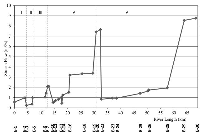
**Figure 5**. Stream Flow profile Chinchina River Basin Data Source: (UNAL- CORPOCALDAS, 2014)
