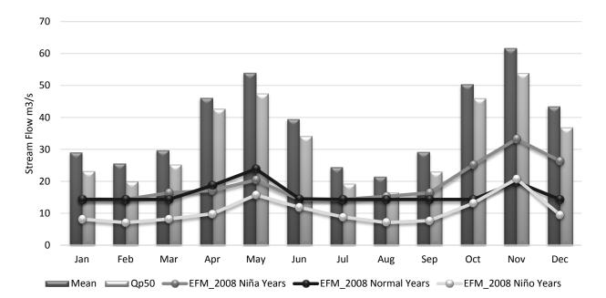
**Figure 8.** Environmental flows in the Chinchina River Basin for different hydrological conditions at El Retiro gauge station.
