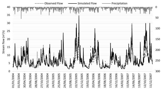
**Figure 8.** Observed and simulated discharges using TETIS model during the validation process, (2004-2007) at Sancancio gauge station.
