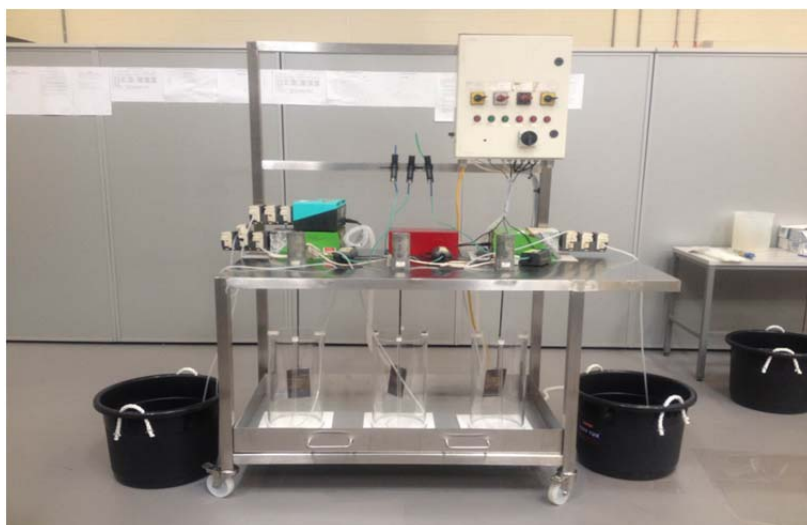
Figure 3: Laboratory-scale intermittently aerated sequencing batch reactor experimental unit at NUI Galway
