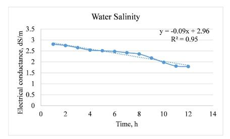
Figure 2. Water electrical conductance measured inside the evaporation zone of the plant.
