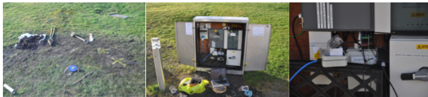
Figure 6: Test site in Falkirk Wheel after the deployment of all subsurface sensor nodes and housing for power supply, getaway and hub.
