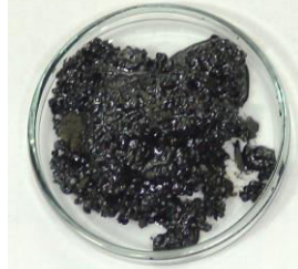
Sand + Fresh Coal Tar
