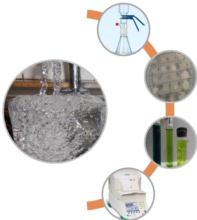
1. Membrane filtration ( $0.22\mu\text{m}$ , 100mL sample)
