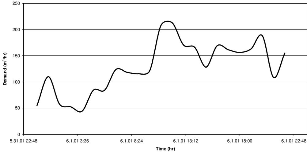
Figure 2. Diurnal curve of June 1, 2001, extracted from SCADA recordings
