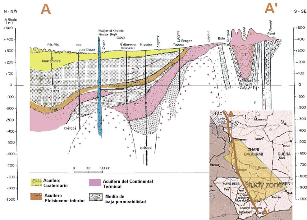
Figure 2. Cross section of the study area showing the existing aquifers (after Schneider, 1989).
