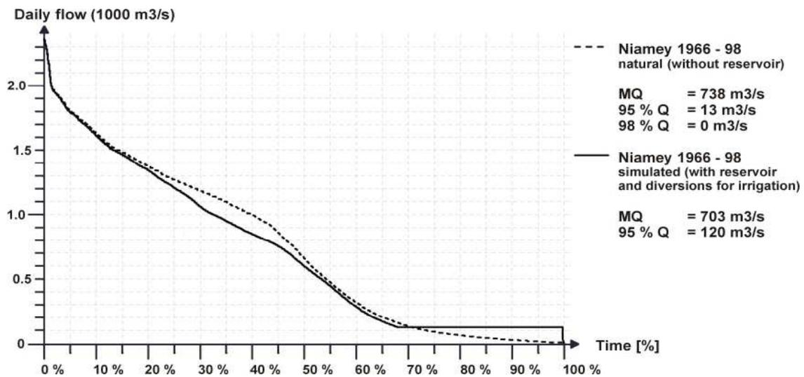
**Fig. 7:** Duration curves of daily flow of River Niger at Niamey (natural and simulated for a required minimum target flow of 120 m<sup>3</sup>/s)
