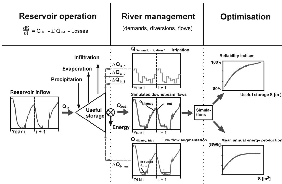
**Fig. 5:** Structure of new water management model for the river Niger flowing through the Republic of Niger, developed by Meon (Lahmeyer International e.a., 2000)
