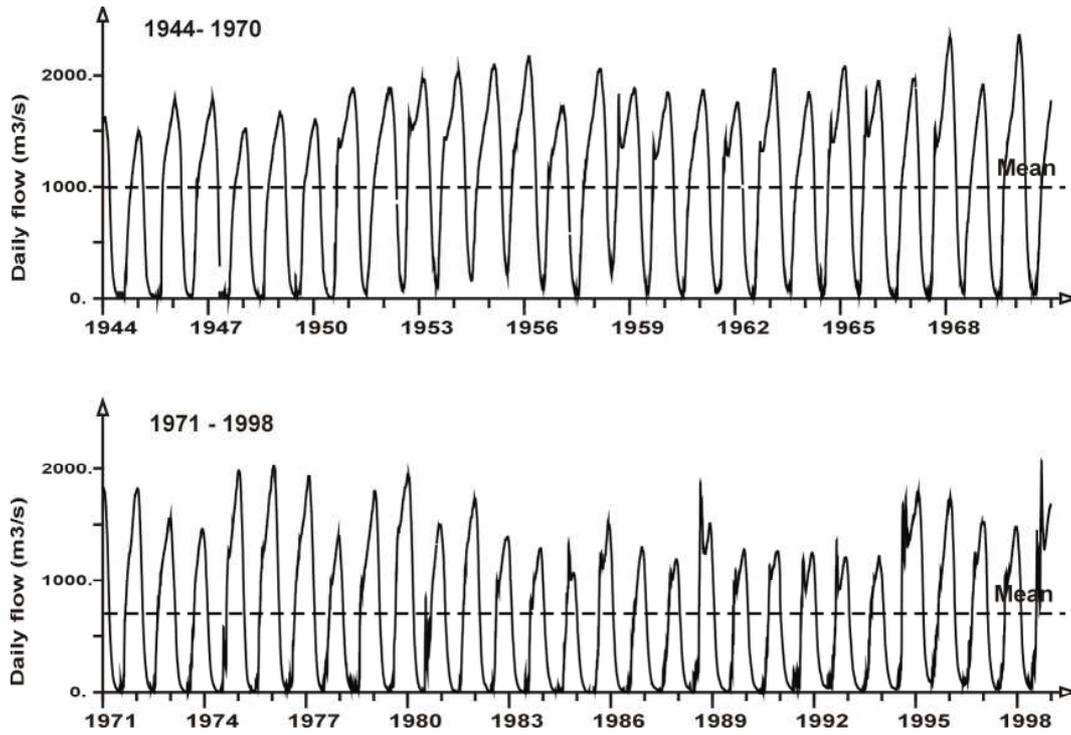
**Fig. 3:** Recorded natural flow of river Niger at Niamey for periods 1944-69 and 1971-98 (processed from raw data obtained from NBA)
