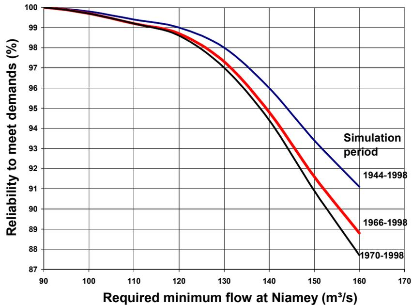
**Fig. 9:** System reliability in dependence on the simulation period
