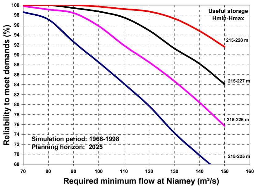
**Fig. 8:** System reliability in dependence on the size of the useful storage and the required minimum flow at Niamey; based on numerous simulations of the reservoir-river system
