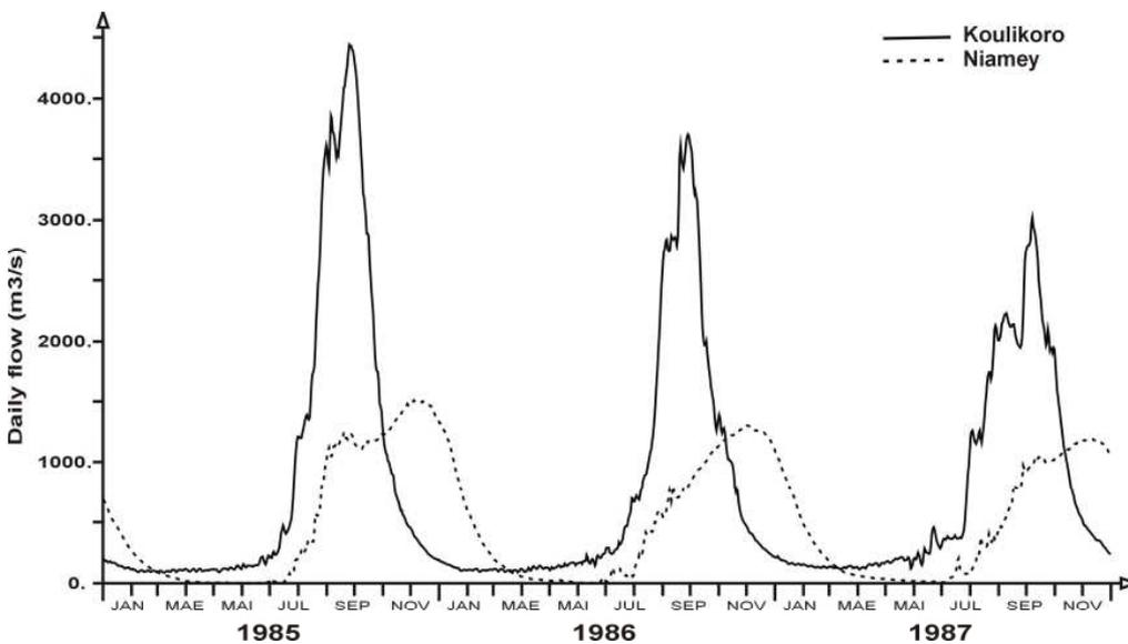
**Fig. 2:** Hydrograph recorded at Koulikoro (upstream of the Inner Niger Delta) and at Niamey during a dry period (source of raw data:NBA)
