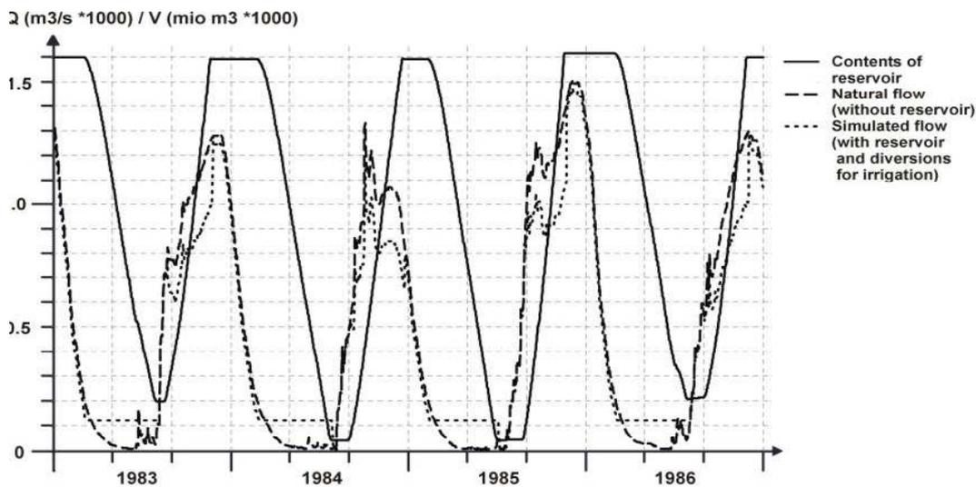
**Fig. 6:** Excerpt of simulation: contents of reservoir and corresponding flow of river Niger at Niamey for a required minimum target flow at Niamey of  $120 \text{ m}^3/\text{s}$
