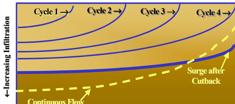
Fig. 5: Surge irrigation: Water percolation in surge and continuous flow
