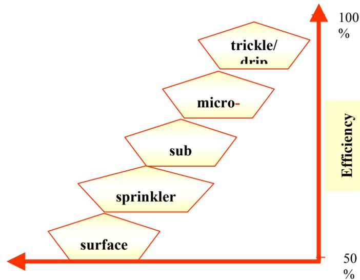
Fig. 4: The five basic methods of applying water to the soil
