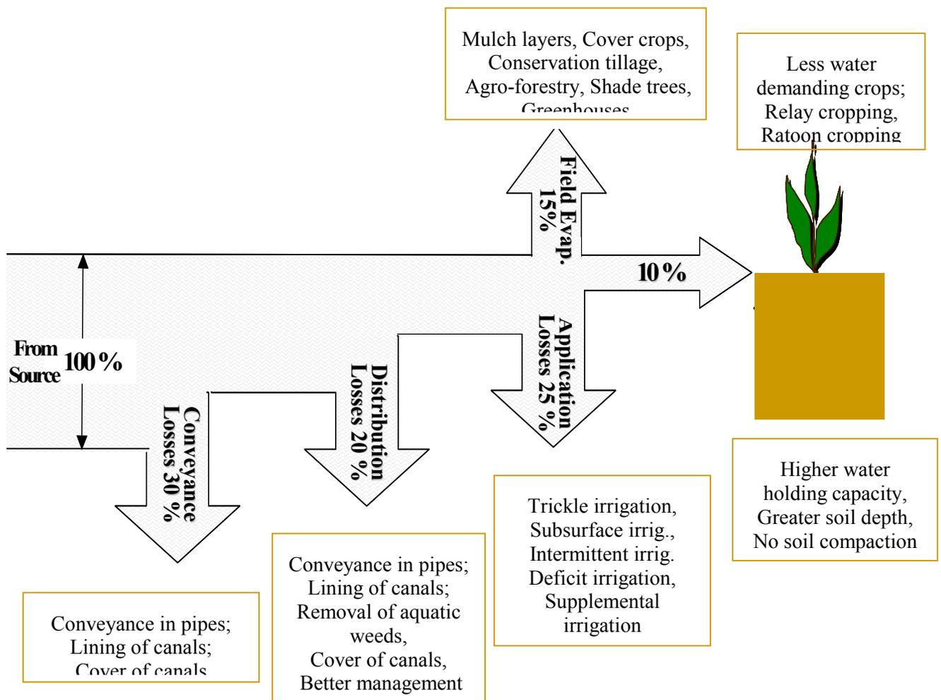
Fig. 3 : Average losses in large irrigation schemes and techniques to arrive at a higher irrigation water efficiency
