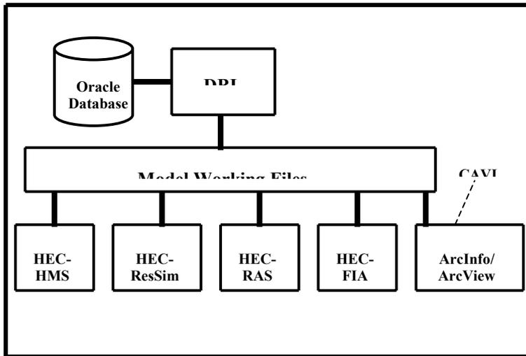
**Figure 4.** CWMS models integration schematic.
