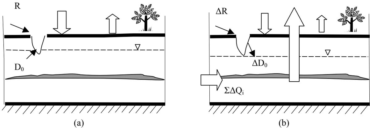
Figure 1. The water budget of a multi-aquifer system: (a) virgin conditions; (b) after pumping begins.
