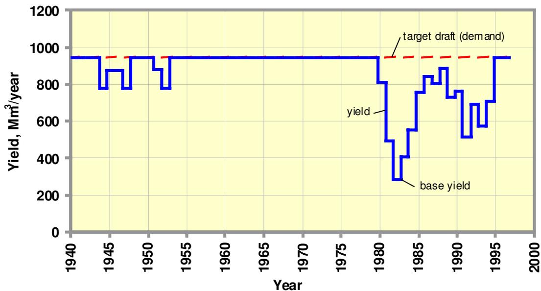
**Figure 2.** Simulated annual yield from the reservoir Bin El Ouidane based on hydrologic data for the period 1939-97, and a target draft of 945 Mm<sup>3</sup>/year
