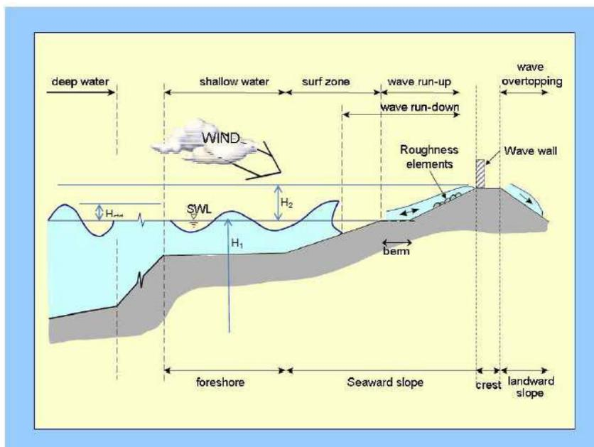
the parameters used in the overtopping computation. The height  $H_1$  refers to the storm surge level and it should be noted that the additional freeboard  $H_2$  required is more than the maximum level of the wave crests.  $H_2$  may be reduced by reducing the river facing slope of the embankment and/or increasing the surface roughness.
