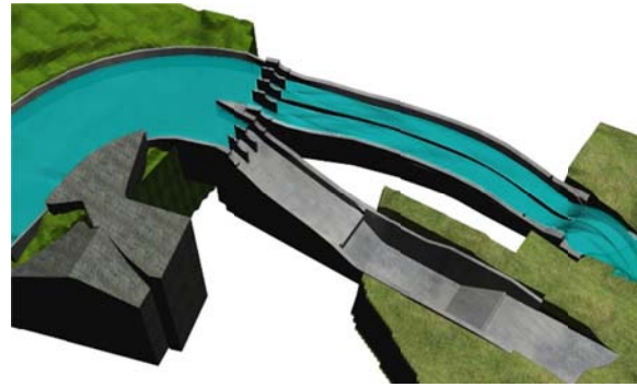
Figure 4. Simulation of the emergency spillway of the Netzahualcoyotl dam
